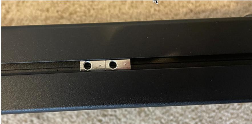
3. Tighten the adapter and use set screws to attach the adapter to the cage nuts in the top of the ticker.
